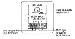
Input terminal of the SF-60 is divided into Low and Mid/High frequencies as the SF-60 is a 2-way multiamplifier driving system.
