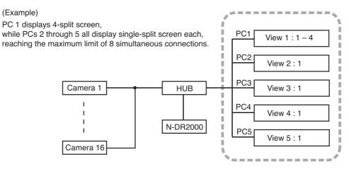
Allows playback of up to 8 views simultaneously.
