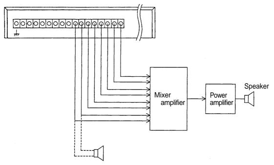
It is also possible to directly connect a high-impedance speaker to these terminals when a high sound volume is not required.
