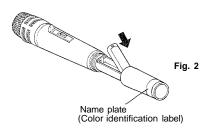
Replace the microphone grip by sliding the grip upward and hand tightening the grip in a clockwise position.
