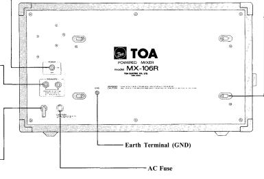
utilized. Operation of the MX-106R with proper grounding techniques will result in less system noise and greatly reduced shock hazard. Warning - To avoid possible equipment damage and/or personnel injury, the fuse should always be replaced with same type and rating. Using improper fuses will also void the warranCord Wrap
