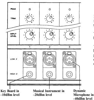
If the trim control is set as shown in the left figure, the input level controls can be set to the same position.
