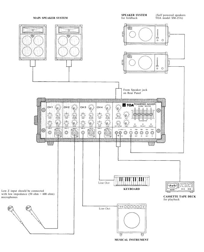
Generally speaking, there are two rules to follow when connecting equipment outputs to the inputs of other equipment.
