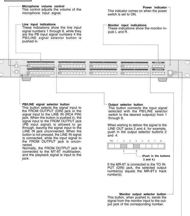
**Power switch** Pressing this switch turns power on. To turn power off, press the switch again.
